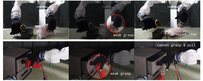
Fig. 7. State-as-Action Failure. Policies trained with measured joint states as action labels produce weak grasps and fail to hold onto objects. Top: the baseline drops the package when presenting it to the scanner. Bottom: the baseline cannot retain the laundry once it begins to pull the drawer open.
